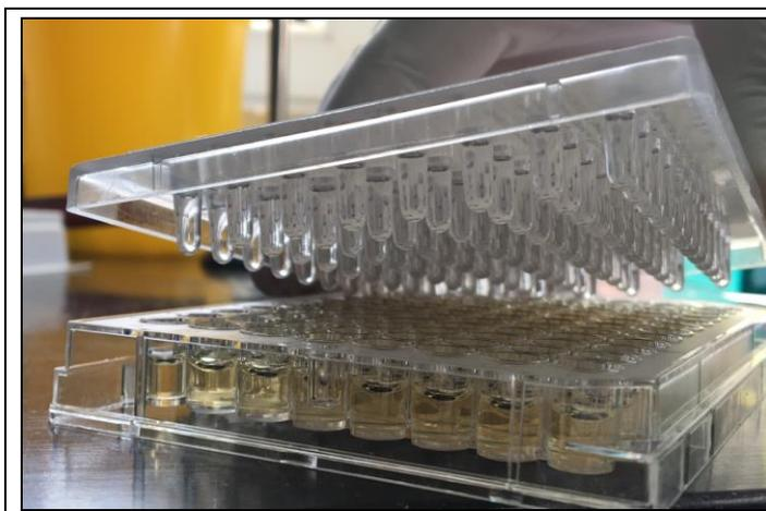
**Figure 1.** Biofilm inoculator with a 96-well plate with peg lids (Innovotech, Inc., Edmonton, AB, Canada). The MBEC biofilm inoculator has a lid with 96 pegs and a base with 96 individual wells. Biofilm grow and established on the peg lid.
