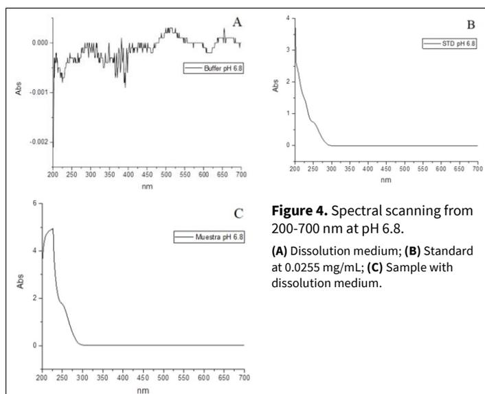
**Figure 4.** Spectral scanning from 200-700 nm at pH 6.8. (A) Dissolution medium; (B) Standard at 0.0255 mg/mL; (C) Sample with dissolution medium.
