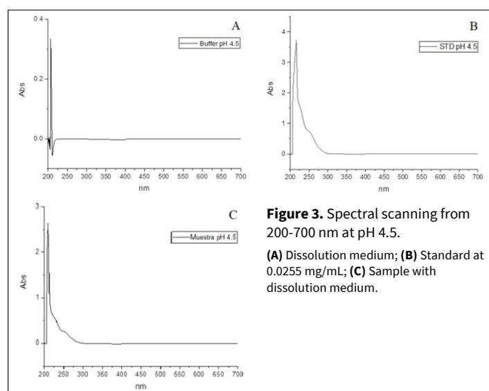
**Figure 3.** Spectral scanning from 200-700 nm at pH 4.5. (A) Dissolution medium; (B) Standard at 0.0255 mg/mL; (C) Sample with dissolution medium.
