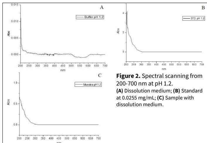
**Figure 2.** Spectral scanning from 200-700 nm at pH 1.2. (A) Dissolution medium; (B) Standard at 0.0255 mg/mL; (C) Sample with dissolution medium.
