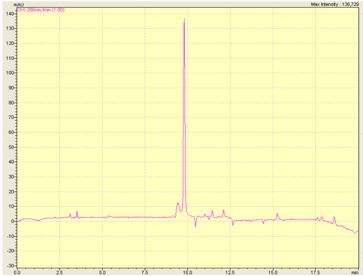
S2. Chromatogram for the HPLC separation of 2 . Retention time 9.79 min.
