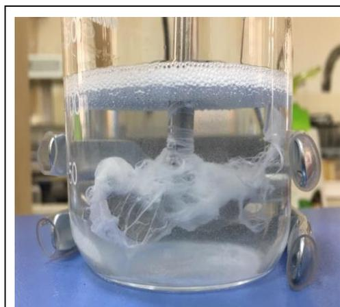
**Figure 1.** Dispersion of CAB methanol solution in water containing PVA.
