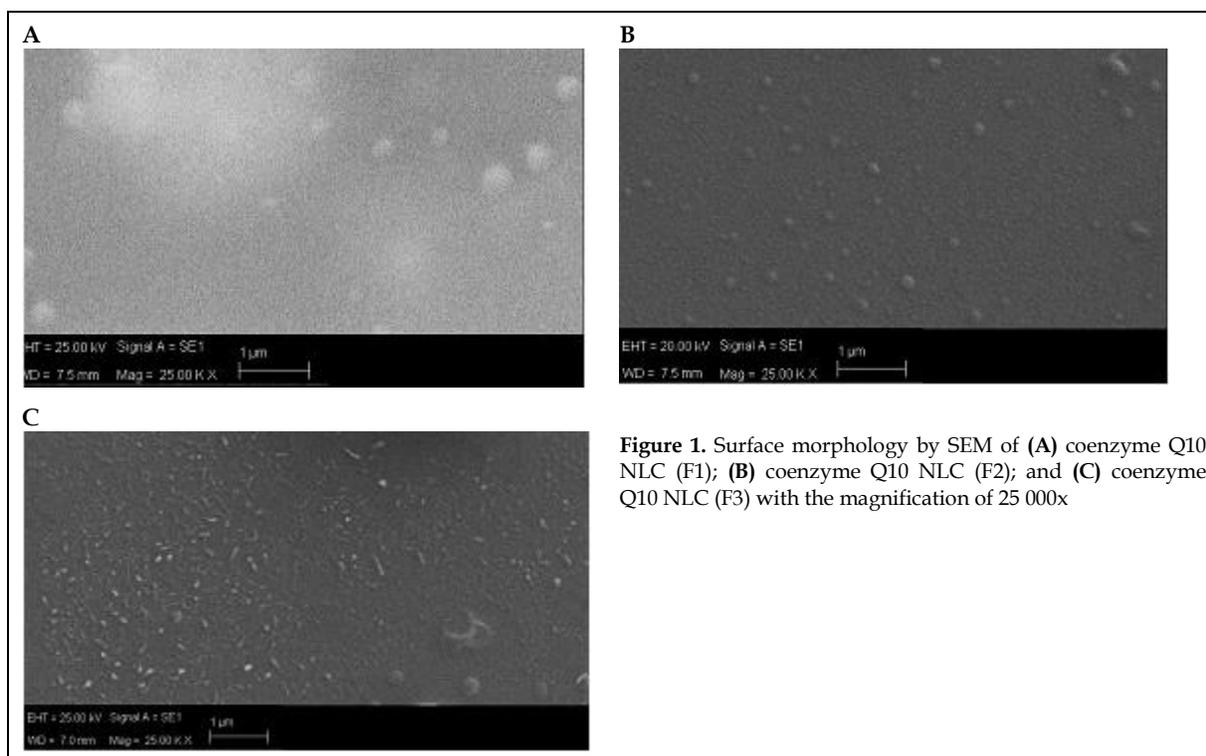
**Figure 1.** Surface morphology by SEM of (A) coenzyme Q10 NLC (F1); (B) coenzyme Q10 NLC (F2); and (C) coenzyme Q10 NLC (F3) with the magnification of 25 000x
